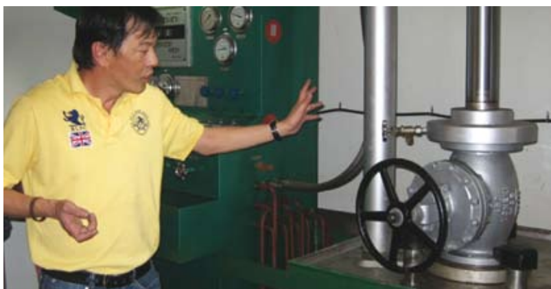
Figure 5: Mr. Lim demonstrating how a valve is tested
